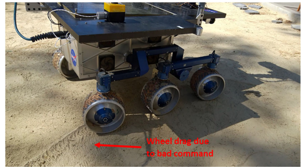
FIGURE 17 A simulated software error leading to an incorrect steering angle [Color figure can be viewed at wileyonlinelibrary.com ]
